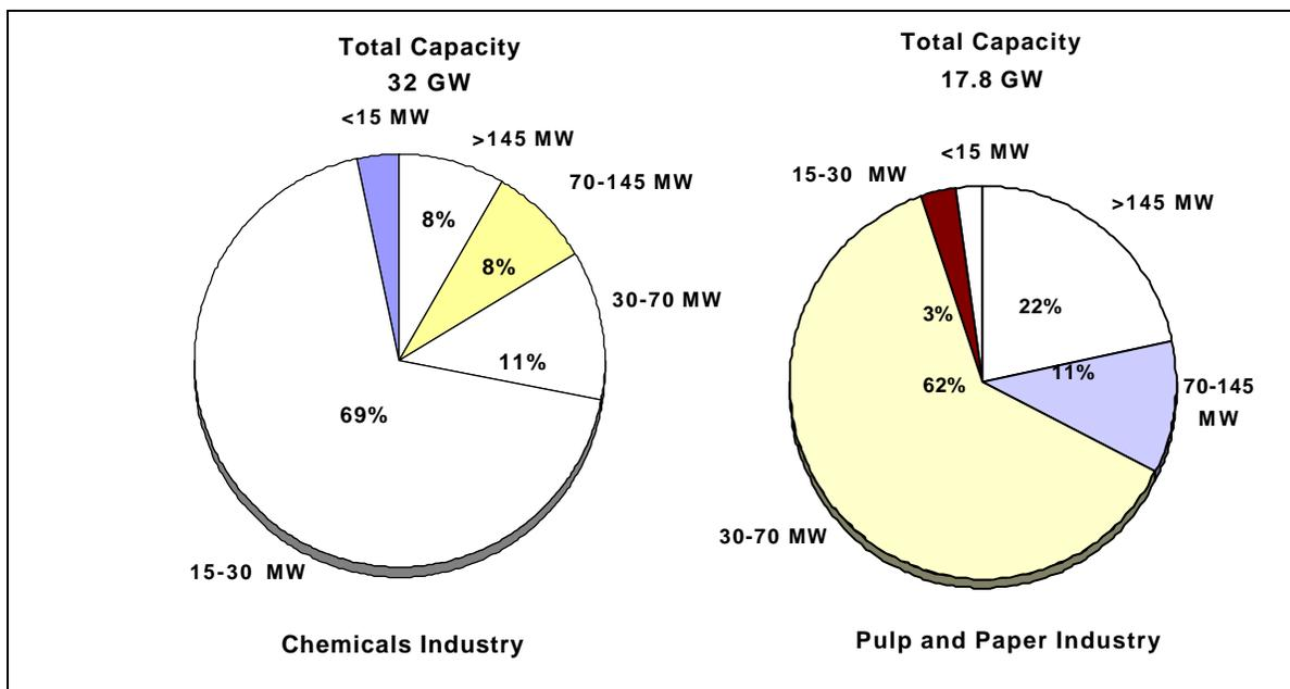
Figure 1. Capacity Distribution of the Remaining CHP Potential
